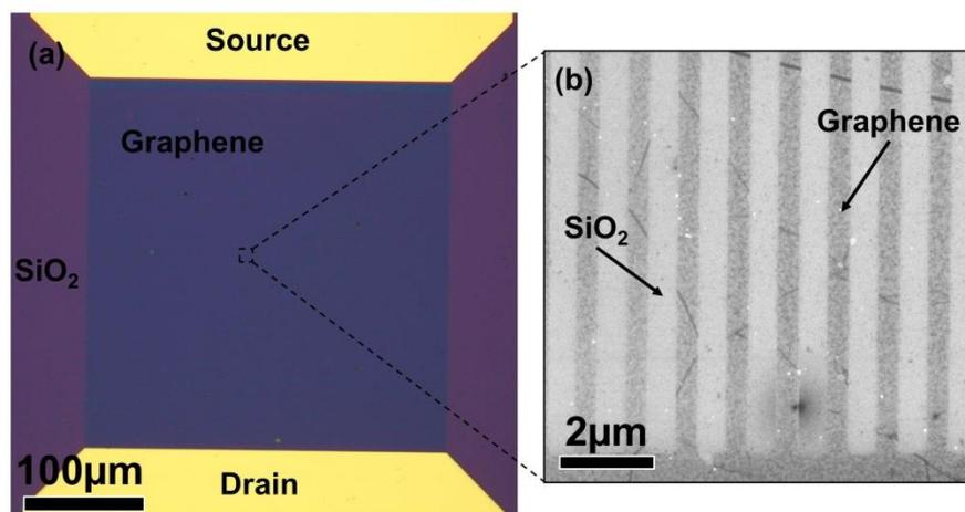
Figure 2: (a) Optical and (b) SEM image of graphene nanoribbon array device.
